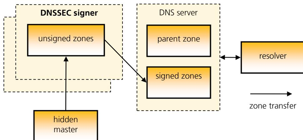
Figure 2.2 Test setup for DNSSEC signers used as a "signer-in-the-middle".
