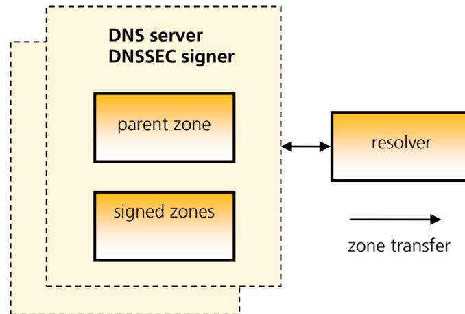
Figure 2.1 Test setup for the IPAM systems and DNS servers.
